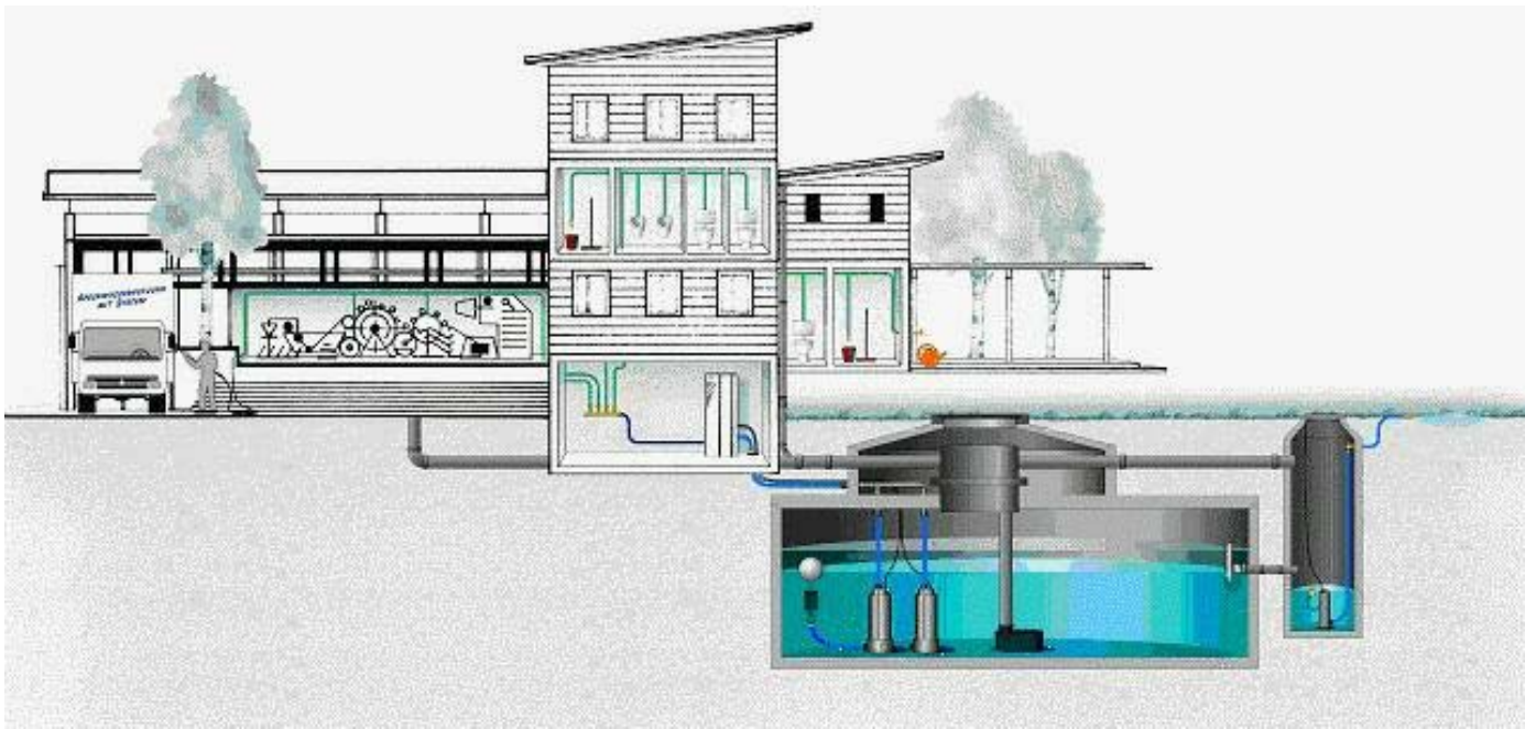
RAINBARREL / CISTERN HARVESTING FOR RE-USE
